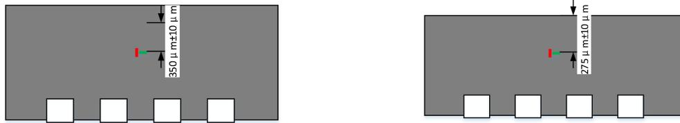
Figure 7-2. The relative position of sensitive area in the QFN3x3 16-Pin package
